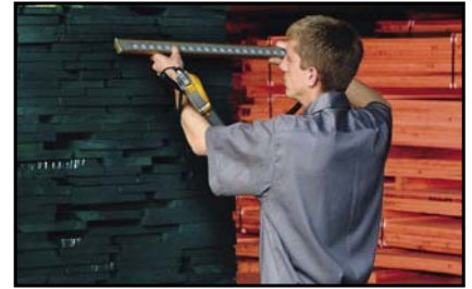
An electronic tally stick attached to the handheld data collection device speeds the job of end tallying lumber.
